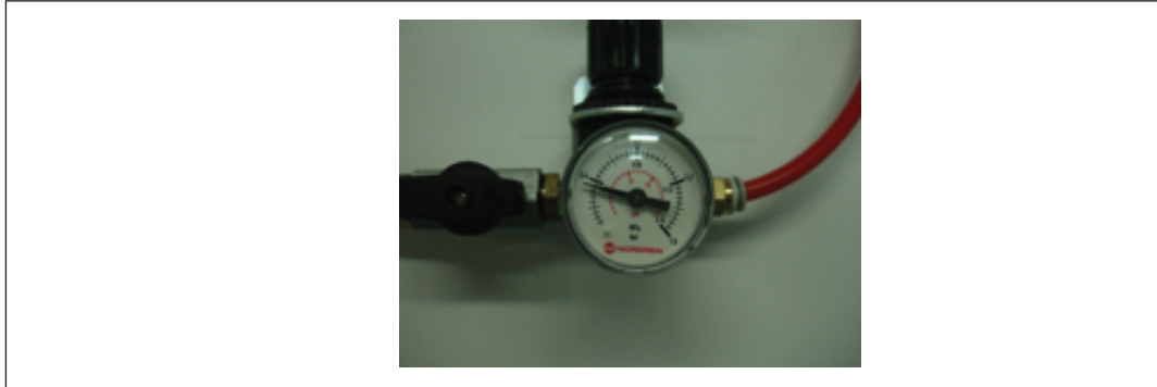
Fig. 4-8: In-line pressure regulator
